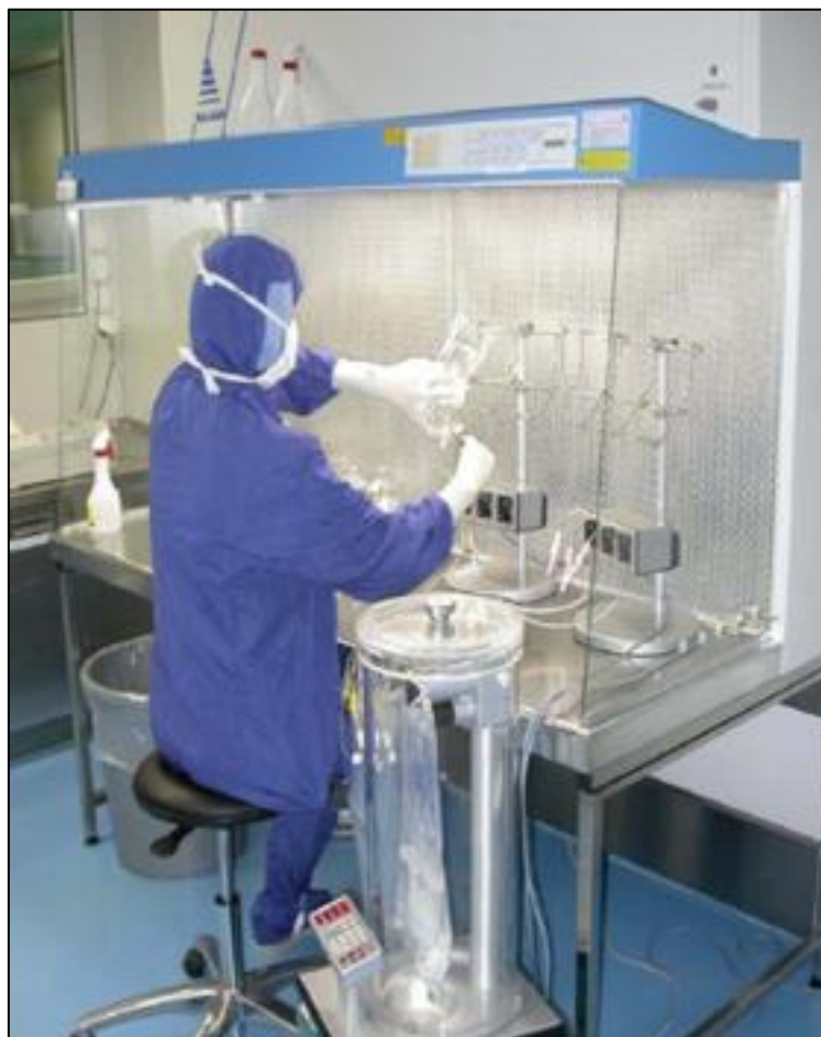
Fig. 4 Aseptic PN compounding in a laminar air flow (LAF) cabinet using a (vacuum) filling machine
